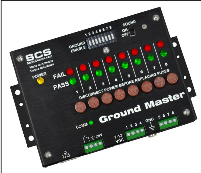
Figure 1. SCS 770044 Ground Master Monitor
